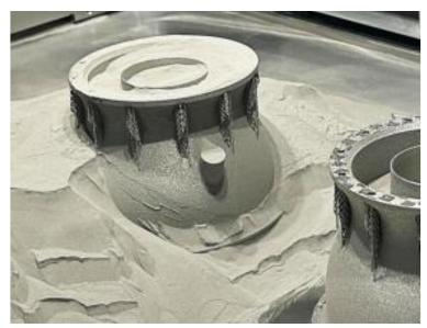
Printed Engine Parts in the Printing Chamber
