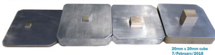
Progression of simple parts printed slowly on the MFP / LFP Proof of Concept Printer
