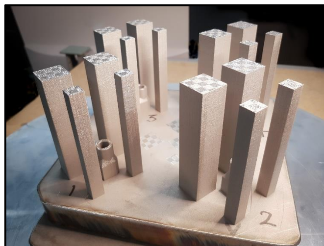
Fig 2: Tensile Bars printed at high laser power
