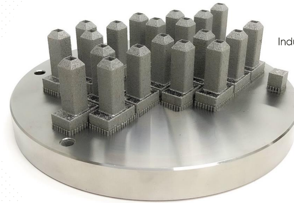
Gland followers commonly used in resources sector pumping systems printed in 316 stainless steel
