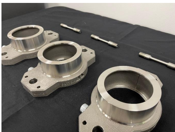
Gland followers (L) and large valve trim (R) printed using 4-laser 1.5kW parameter sets on the RMP-1 Beta
